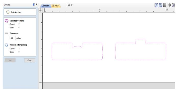
Sometimes it will be necessary to use the join vectors command under the Edit>Join Vectors menu. Even if your vectors were connected as one shape when you exported, they may come into Vcarve segmented and need to be joined to closed shapes.
