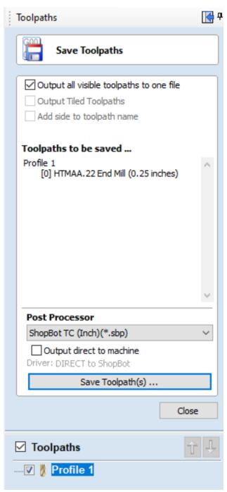
Under Toolpath Operations, Click Save Toolpath, the icon that looks like a floppy disk. Because we're using the same tool for all cuts, we can click the "Save all visible toolpaths to one file" button, but make sure that the cuts are listed in the correct order above this box before saving as such. Make sure Post Processor is in "Shopbot TC (inch)(\*.sbp)" Click Save Toolpath. Name it. Also, go to File:Save As and save your file as a Vcarve file for easy editing if necessary.
