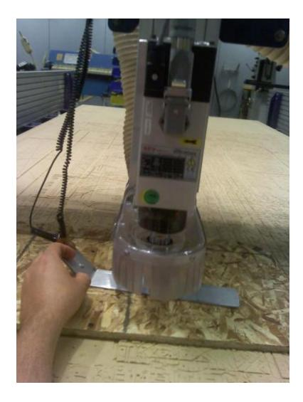
In the Shopbot Console, go to menu "Cuts" and run command "C2 - Zero Z axis w/ ZZero Plate." Click OK. The machine automatically zeros the Z axis. Click OK after. Return the metal plate to its holder on the side of the spindle.
