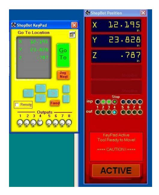
Move the tool over the material. Lower the tool until it is a few inches away from the material. Remove the long metal plate from the side of the spindle holder and lay it flat on your stock, under the tool.
