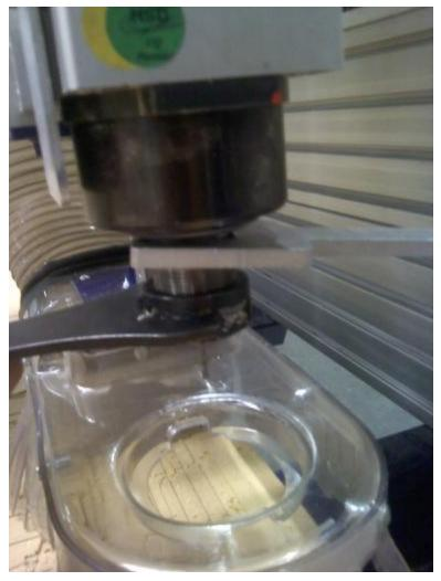
Raise the dust collection skirt up over the tool. There is a thumb screw between the 2 springs behind the spindle to hold it in place.
