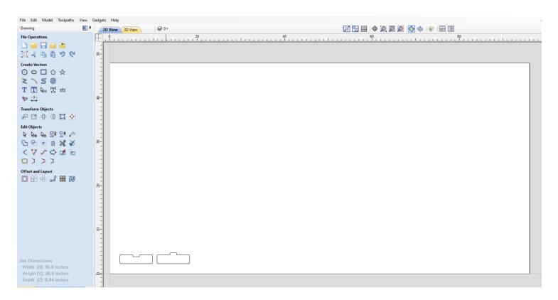
On Drawing screen: Under Edit Vectors Heading: Using the 3rd arrow tool from the left (Move, Scale, Rotate Selection) drag to select your entire part and fit it inside the white box that represents your stock. This tool can resize or rotate by dragging square-marked and circle-marked corners, respectively, and move by dragging from the center of the part.
