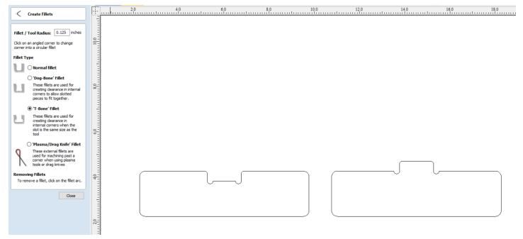
Note: Press fit parts require filleted slots on inside corners. To achieve this, select the fillet tool under Edit Vectors, and select T-Bone Fillet. Input your tool size, and click on two lines to create a fillet between them.
