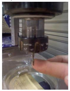
Grab the flat sides of the spindle with a 27 mm wrench. Use the black ER25 Collet Wrench to grab the collet holder. Using both of these, snug the collet holder onto the spindle.
