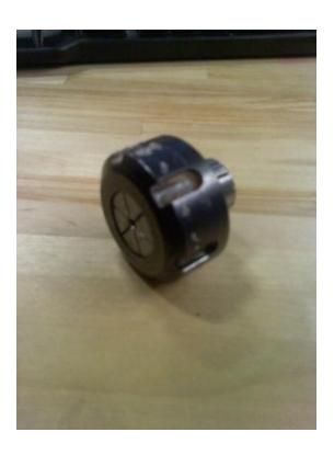
Start to thread the collet holder onto the spindle, one or two threads on. Insert the tool into the hole in the collet. Push it in until the flutes are almost touching the collet, but not. Hand tighten the collet holder on the spindle.
